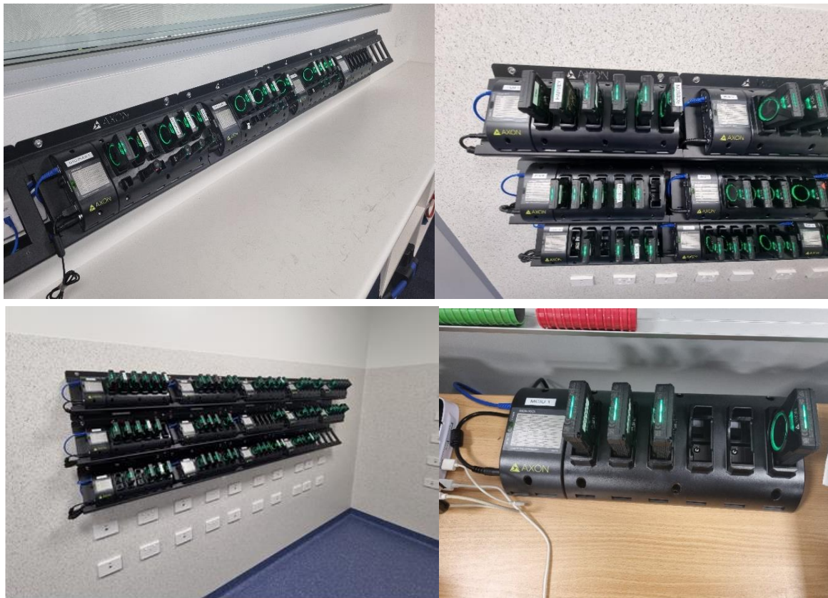
Figure 1.3: NT police BWV Docking Stations – Palmerston police station
